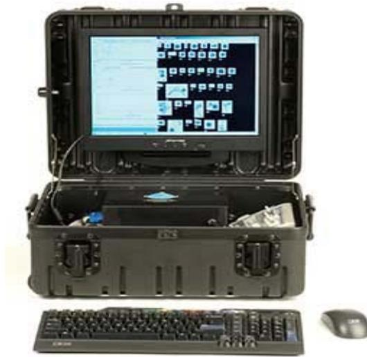
**Figure 1. Portable fluid imaging FlowCAM technique.**
